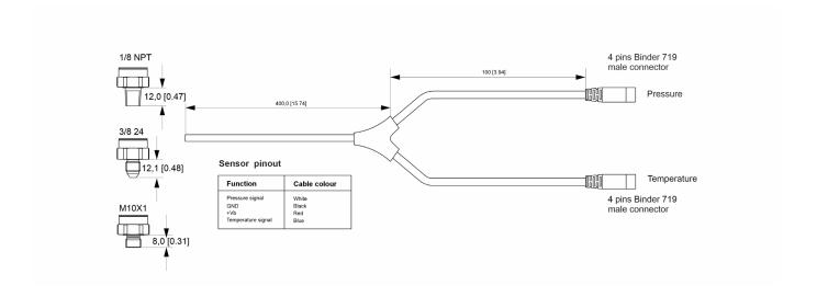
Here below is the cable constructive scheme.
